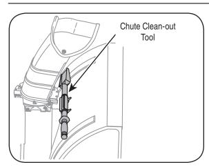
A **chute clean-out tool** is fastened to the top of the auger housing with a mounting clip. The tool is designed to clear a chute assembly of ice and snow.
